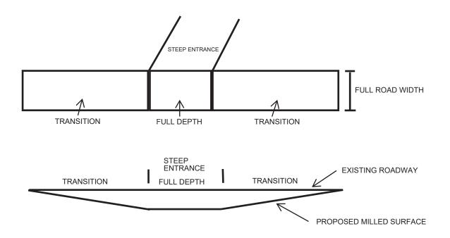
NOTE: THE TRANSITION LENGTH IS BASED ON 100 FT/INCH OF THICKNESS.
